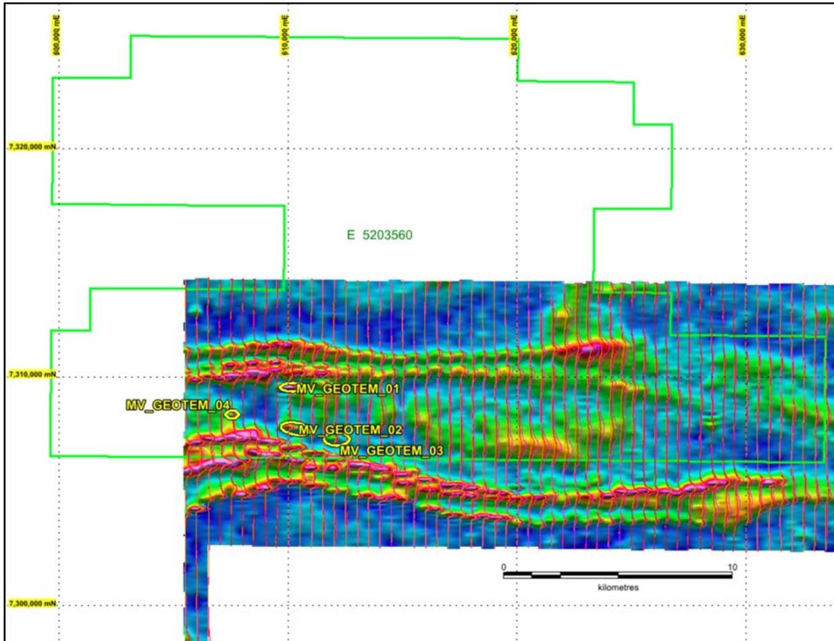
**Figure 2.** Image showing historical airborne EM data from the Mt Vernon Project (GEOTEM Ch20) along with detected anomalies (labelled GEOTEM\_01 to GEOTEM\_04).
