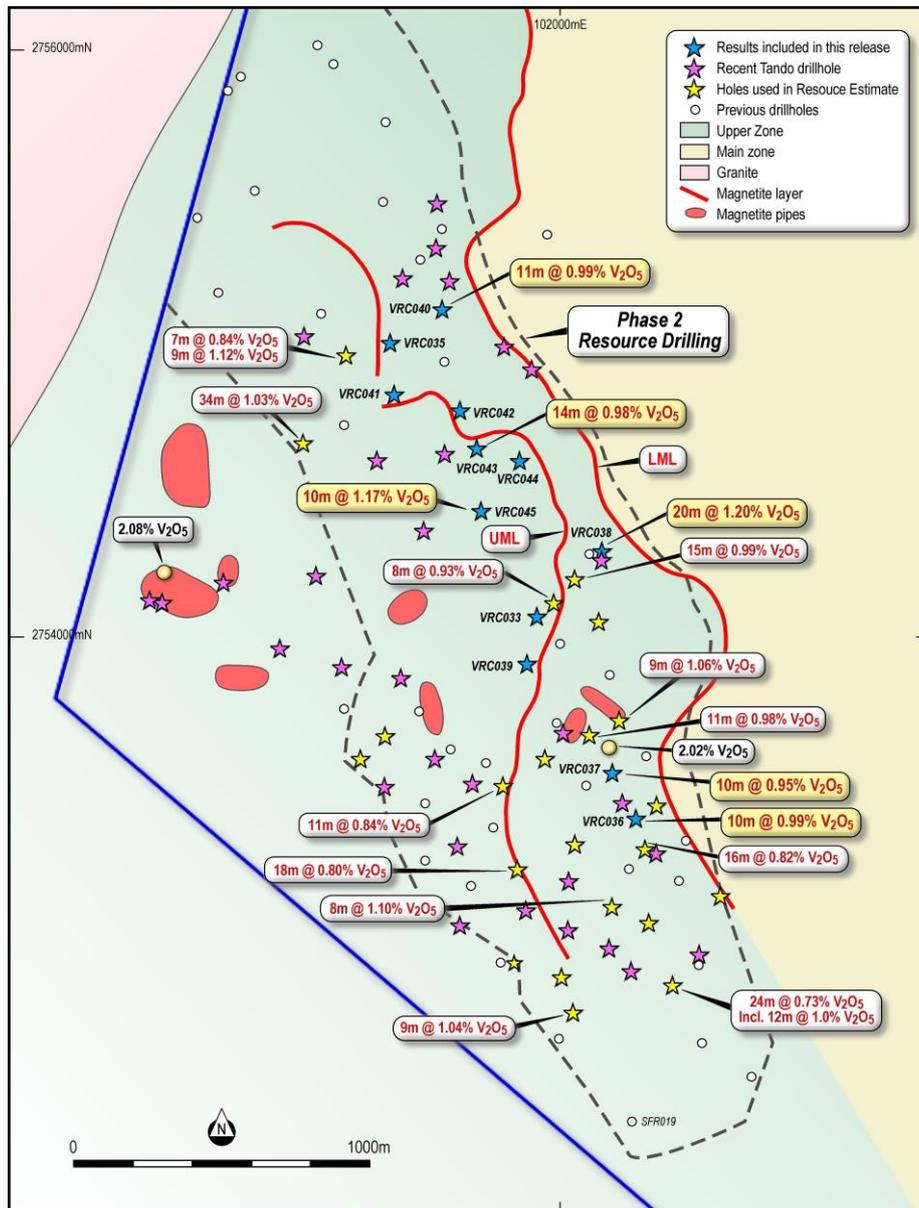
**Figure 1.** Plan showing location of drilling at SPD as well as historical and planned drilling.
